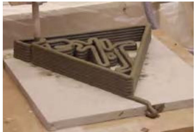
Figure 2: Combination of a robotic arm with the MiniShot system; 3D Sika logo
