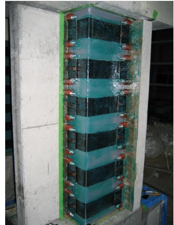
Figure 3.4.5-1 Methods of Wrapping Continuous Fiber Sheets Adopted in Past Researches
