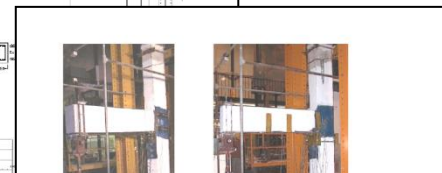
Fig. 17: Tests of external beam-column joints with shear
