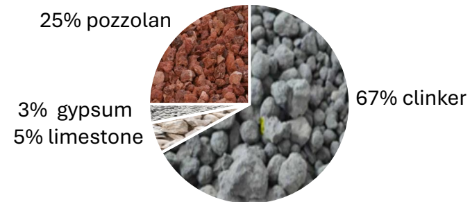
Cement 1P25 – ASTM C595 Clinker, Gypsum, Limestone, and Pozzolan
