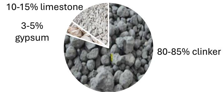
Type 1L - ASTM C595 Clinker, Gypsum and Limestone (higher content)
